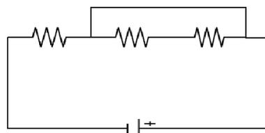
Figure 4. DC circuit question 1: In the following figure all resistors have the same value  $R$  and the voltage of the battery is  $V$ . Find the total current flow through the battery. One way to do this is to trace each possible path from one side of the battery back to the other side.
