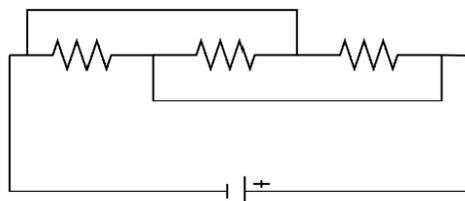
Figure 5. DC circuit question 2: Now, you add one wire to the same circuit as shown. Though there is only one additional wire, there are more paths going from one side of the battery to the other. Find the total current flow through the battery at this time. A similar question was used at a high school Science Olympiad.
