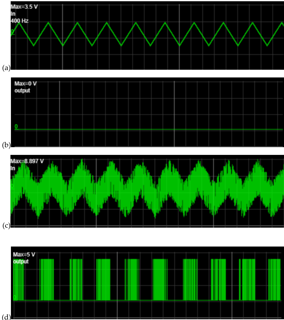
Figure 9. TDG of (a) input without noise (b) output without noise; (c) input with noise (d) output with noise
